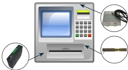
A wire mesh is placed inside the front of the controller and detects drilling in the fascia.
