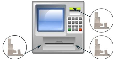
Anti-drilling metal plates are installed on the locations defined according to the manufacturer and the PLC model.
