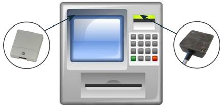
The seismic detector is installed on the upper part of the controller or on a plate fixed under the card reader. If the facade is pierced, the alarm center will immediately receive a signal.
