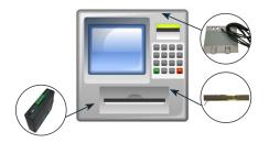
A wire mesh is placed inside the front of the controller and detects drilling in the facia.
