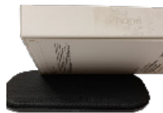
Align top phone label (back of Tracker) with center of charger. An LED light indicates power is being supplied to the pad
