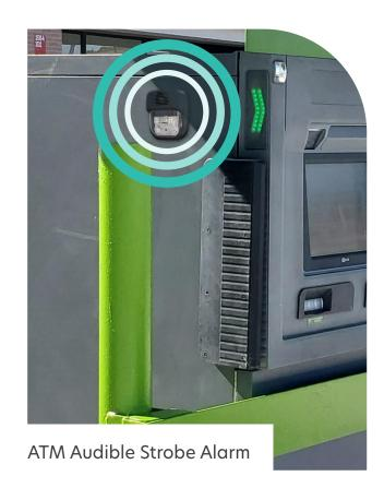
The ATM Security Barrier can be used alongside the Cennox ATM Audible Strobe Alarm to provide an additional layer of security. Both alarms connect to the ATM's alarm panel and provide immediate alerts to the bank when potential threats are detected.
